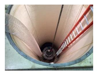
The TRIGA reactor assembly was located in a below-ground 20 foot deep steel reactor pool/tank structure with only vertical access to the core. The reactor assembly contained a graphite-reflected fixed core constructed of aluminum resting on a platform that raises the lower edge of the assembly about 2 feet above the tank floor.
